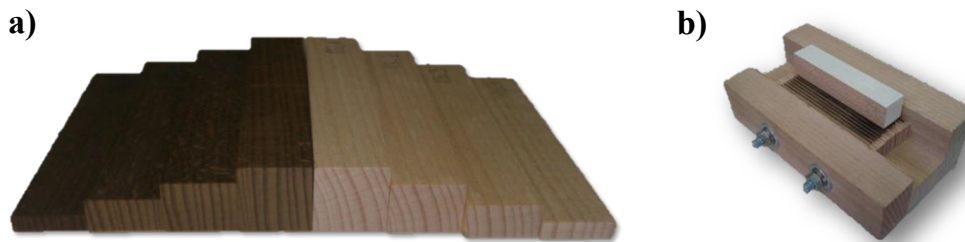
Figure 1: Determination of water vapour diffusivity of thermally modified beech wood by the nonstationary experiment (a) and finite difference method (b).
