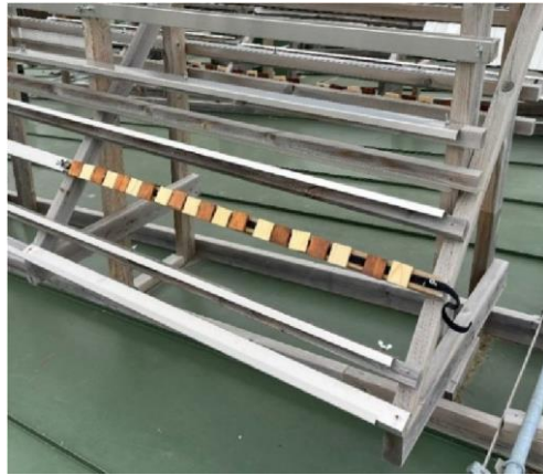
Figure 1: Test site for outdoor weathering test.
