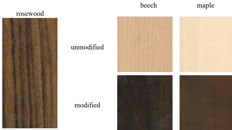
Figure 1: Change of wood colour after a two-step modification (thermal modification and impregnation with PF-resin) and comparison to the wood colour of rosewood
