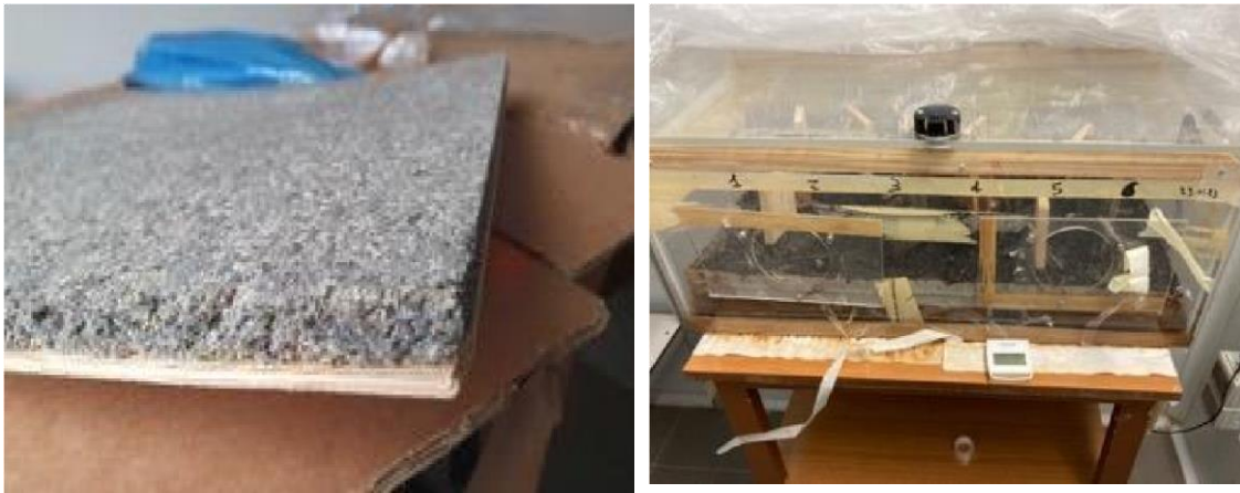
Figure 1: Wood particleboard with encapsulated ethyl palmitate ester as bioPCM processed by the Swedish team for testing the internal bonding (left). A set for testing the susceptibility to mould growth of the bio-composites (right).
