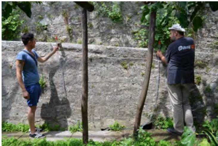
Measurement of the slope of a flume in the upslope terrace at La Malora lemon house.
